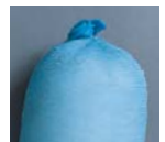
Socks filler expands and gels as liquid is absorbed
